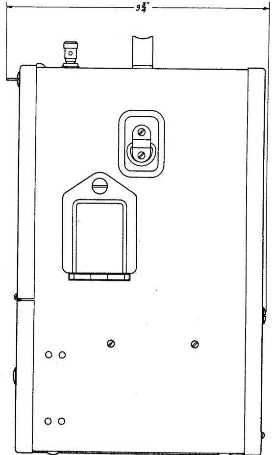
WEIGHT OF CASE WITH TYPE CRR-74028 FREQ. METER WITHOUT BATTERIES 25.5 LBS.
