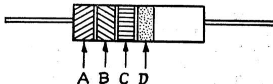
Band A indicates the first significant figure of the resistance of the resistor.
