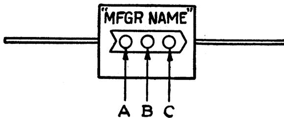
Dot A indicates the first significant figure of the capacitance of the capacitor.
