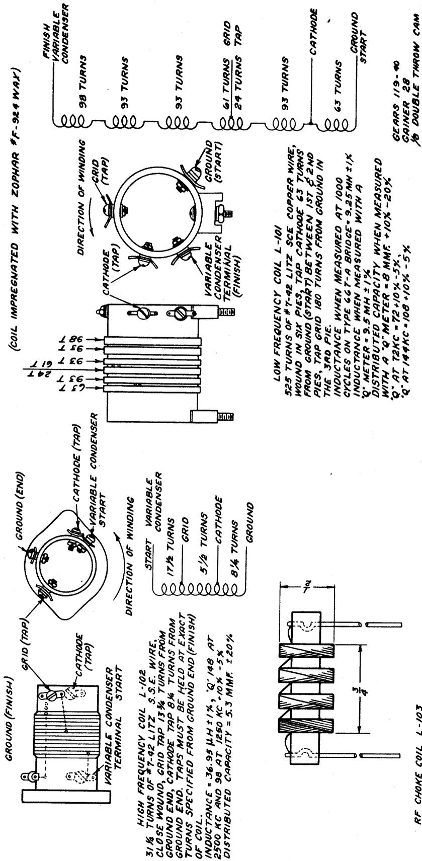
Figure 21. Coil Winding Data
