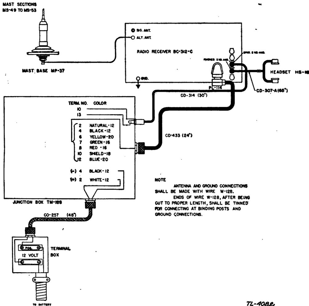
FIGURE 17.—Radio set SCR-210-F, cording diagram.
