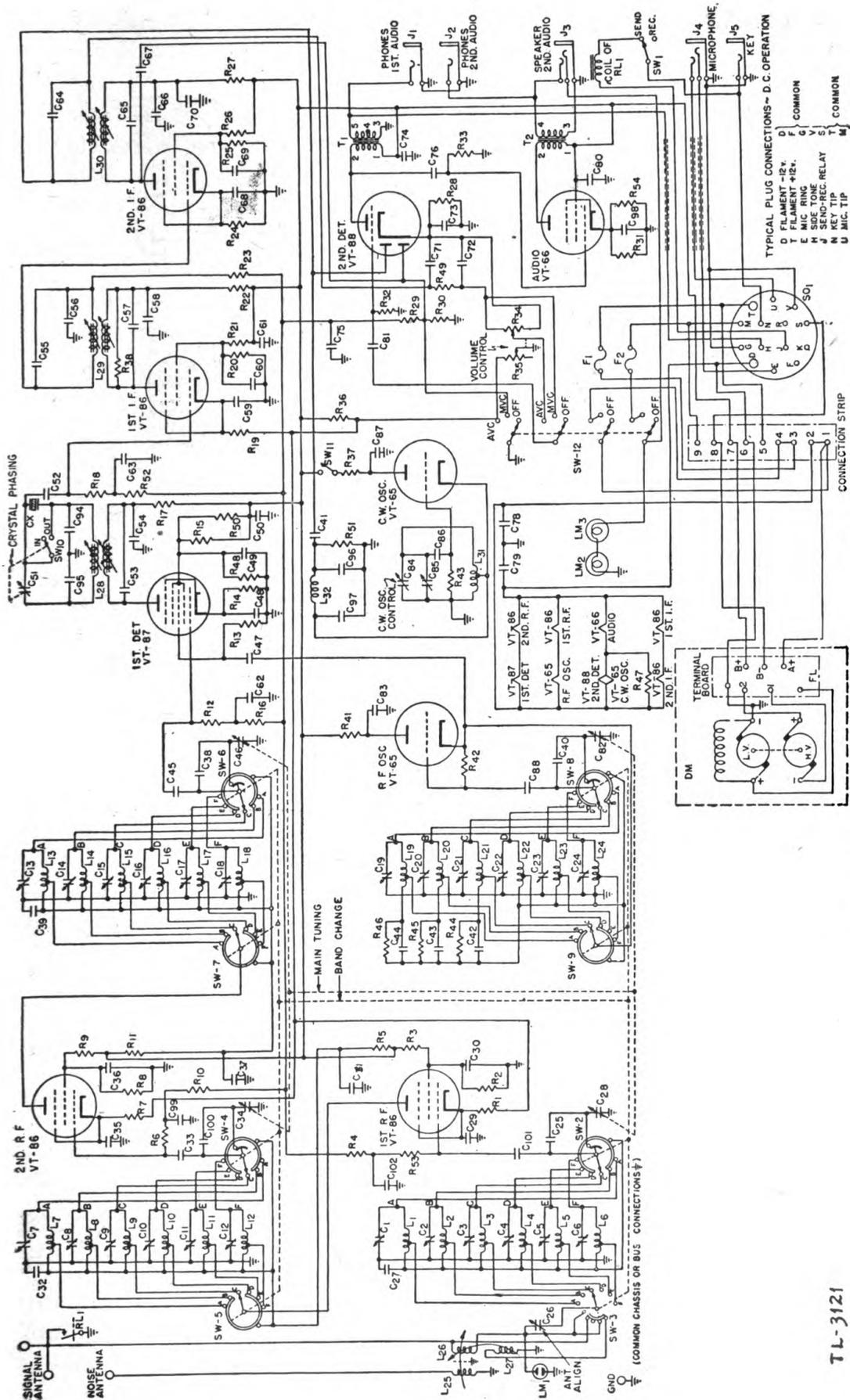
FIGURE 58.—Radio receiver BC-312-C, circuit diagram.
