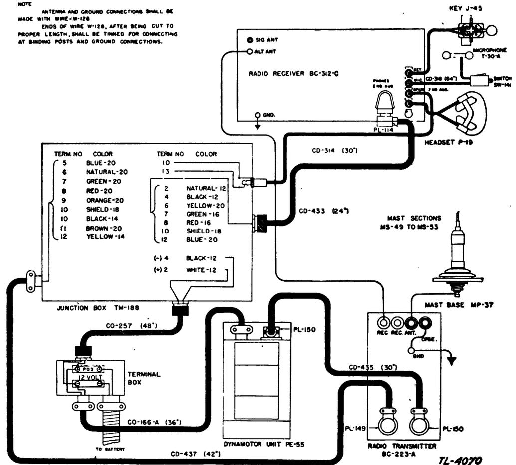
FIGURE 35.—Radio set SCR-245-L, cording diagram.
