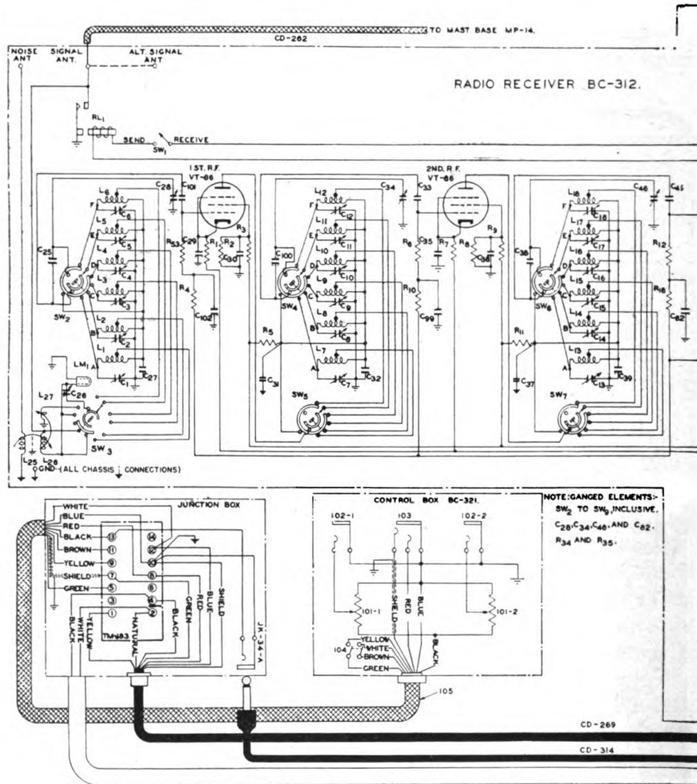
FIGURE 12.—Radio set SCR-210-A, schematic diagram, including
