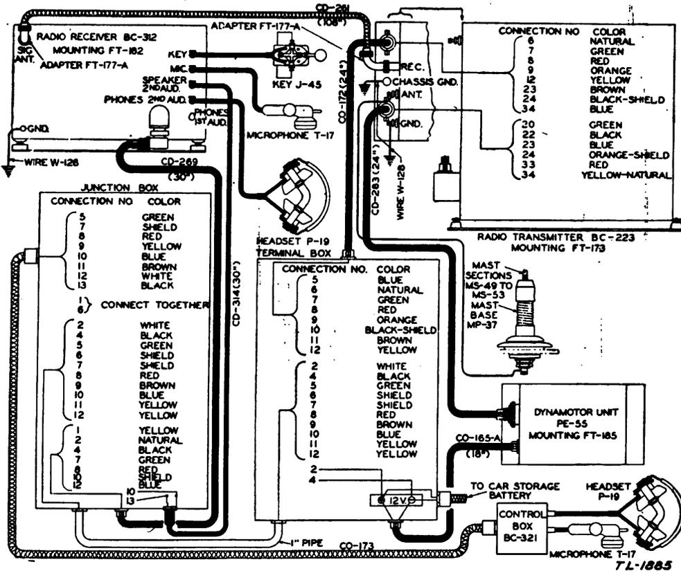
FIGURE 21.—Radio sets SCR-245-A and SCR-245-B, cording diagram.
