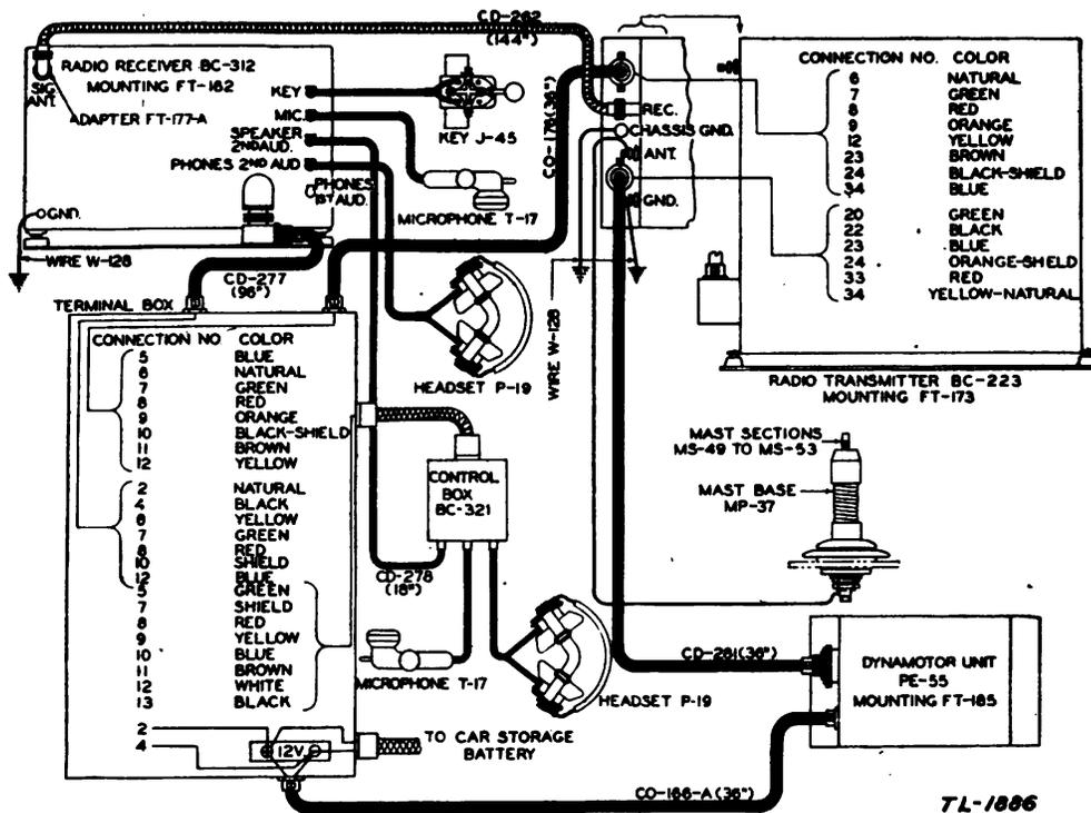
FIGURE 23.—Radio set SCR-245-C, cording diagram.
