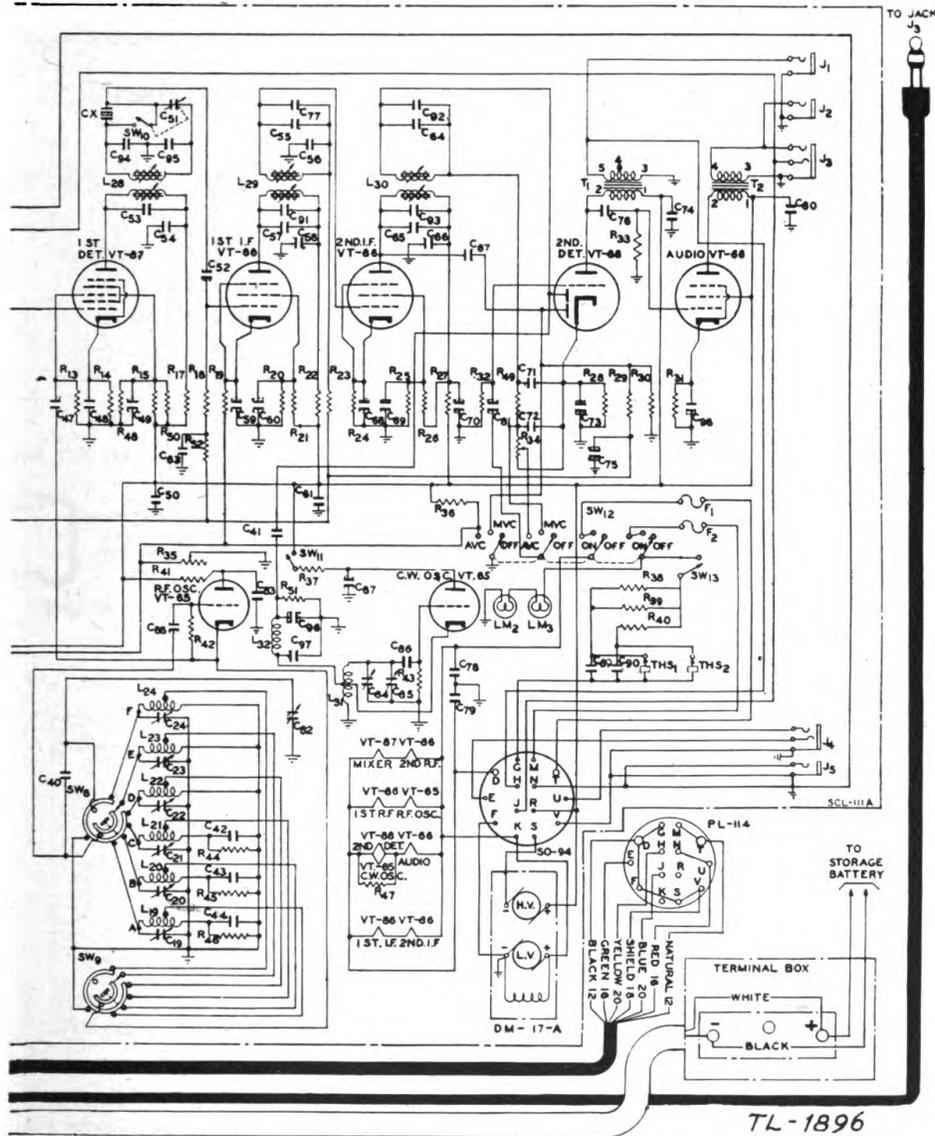
complete schematic diagram of radio receiver BC-312.
