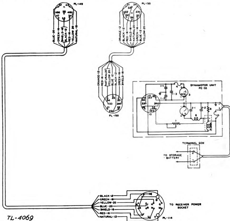
FIGURE 36.—Radio set SCR-245-I, transmitter schematic diagram.
