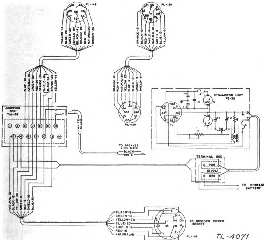
FIGURE 34.—Radio sets SCR-245-K, SCR-245-M, and SCR-245-N, transmitter schematic diagram.
