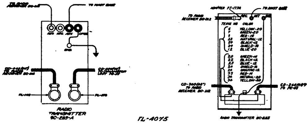
FIGURE 30.—Radio set SCR-245-H, cording diagram.
