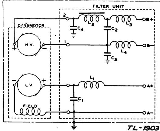
FIGURE 54.—Dynamotor DM-17-A, schematic diagram:
