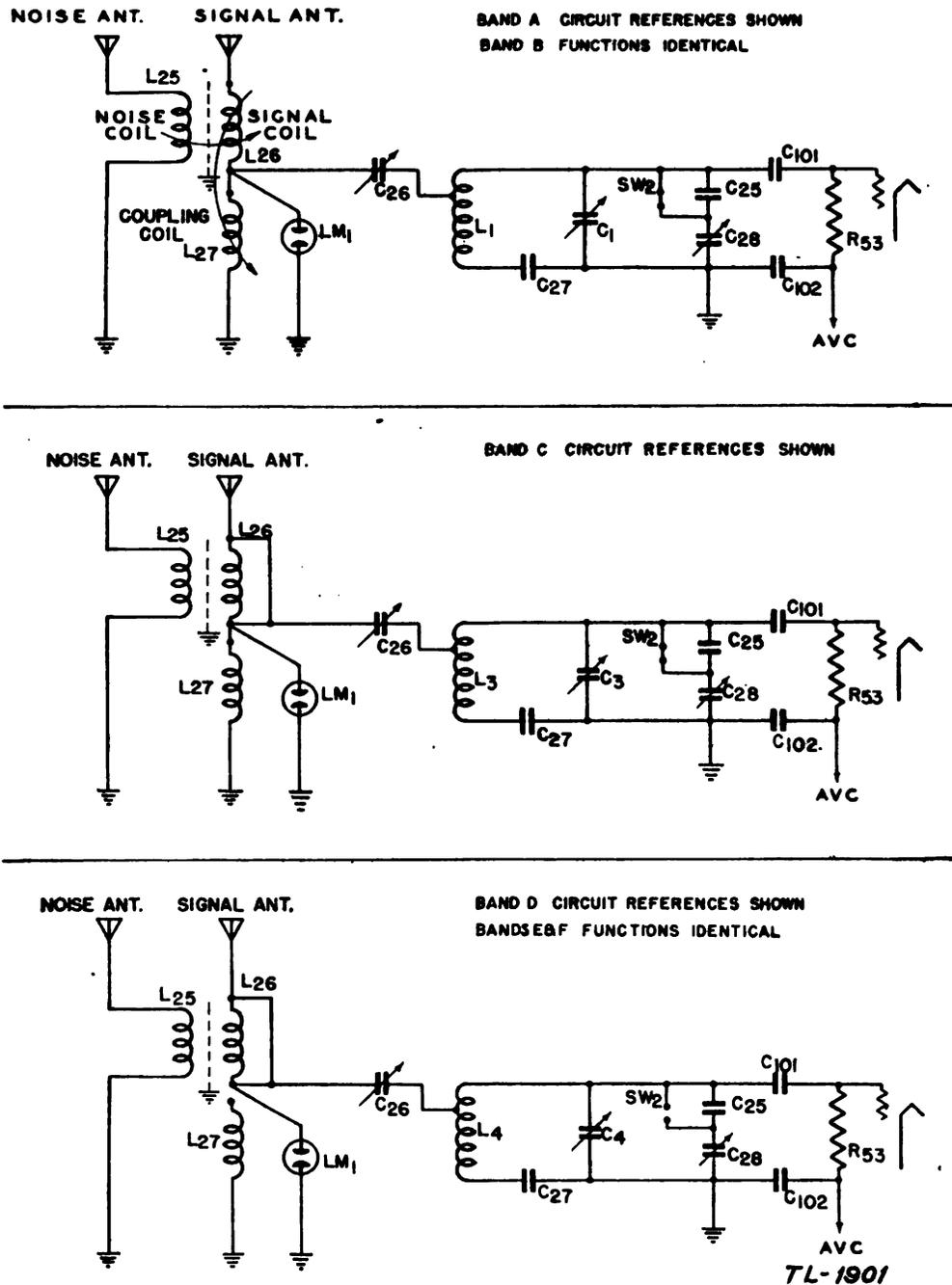
FIGURE 50.—Radio receiver BC-312, antenna circuits, functional diagram.
