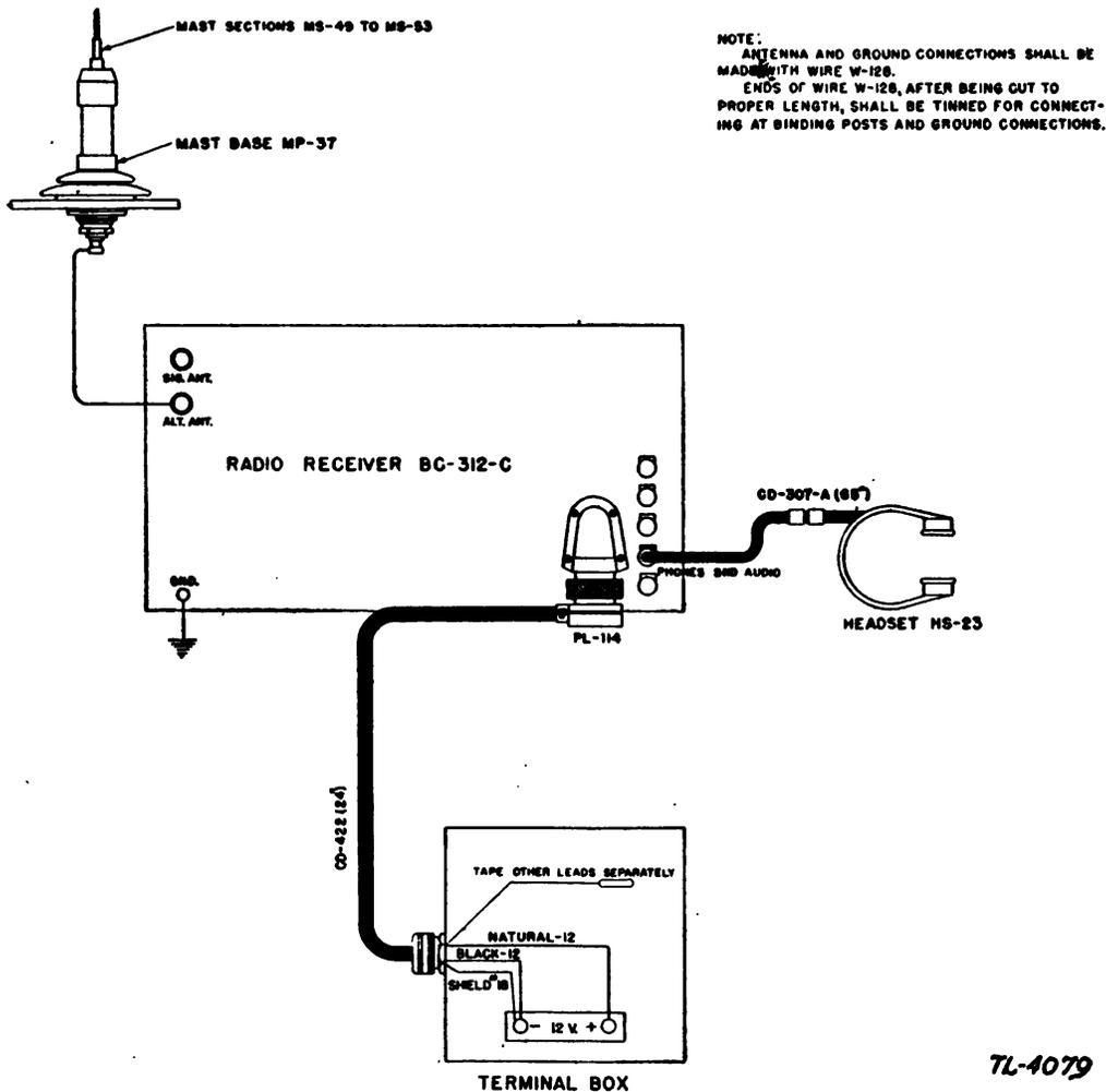
FIGURE 20.—Radio set SCR-210-J, cording diagram.
