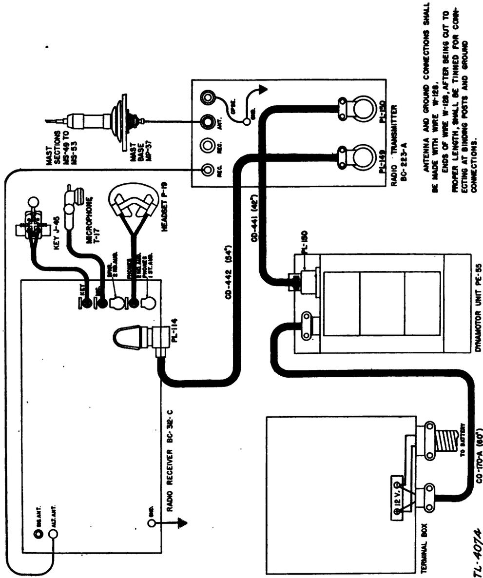
FIGURE 31.—Radio set SCR-245-J, cording diagram.
