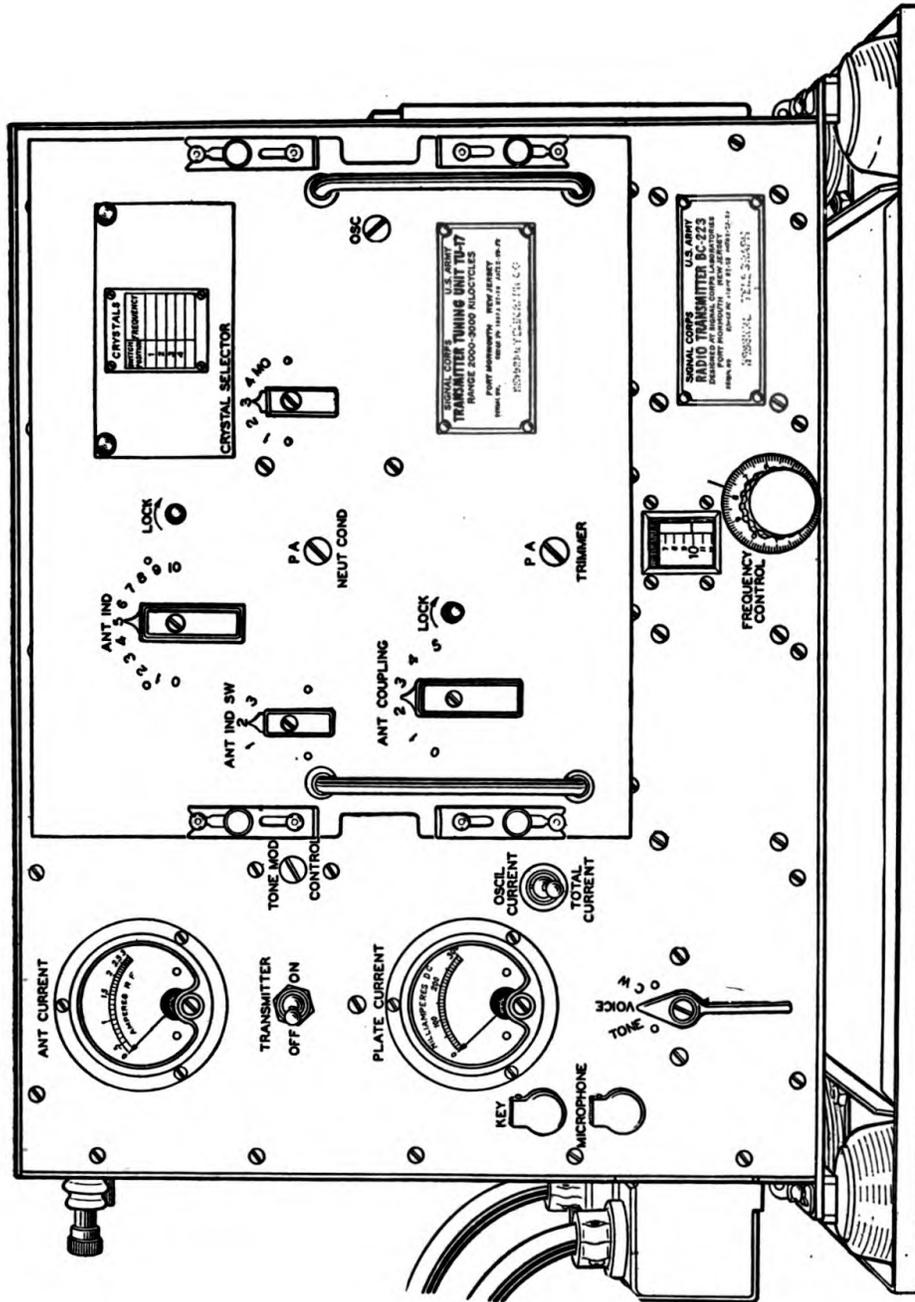
FIGURE 2.—Radio transmitter BC-223 with transmitter tuning unit TU-17 in place, front view. TL-1834
