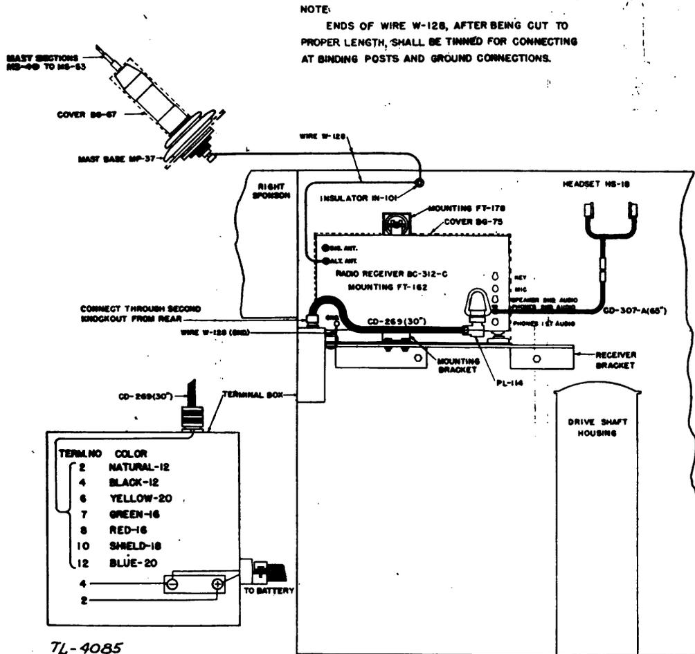
FIGURE 14.—Radio set SCR-210-C, cording diagram.
