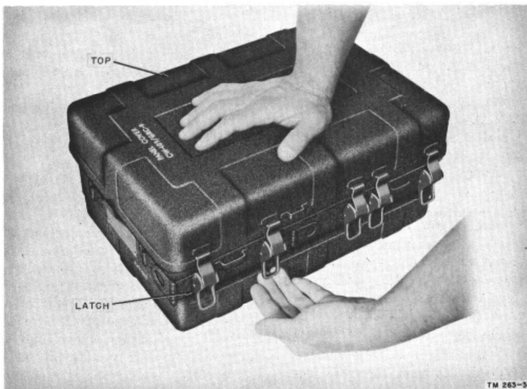
Figure 28. Removing front cover of receiver-transmitter.
