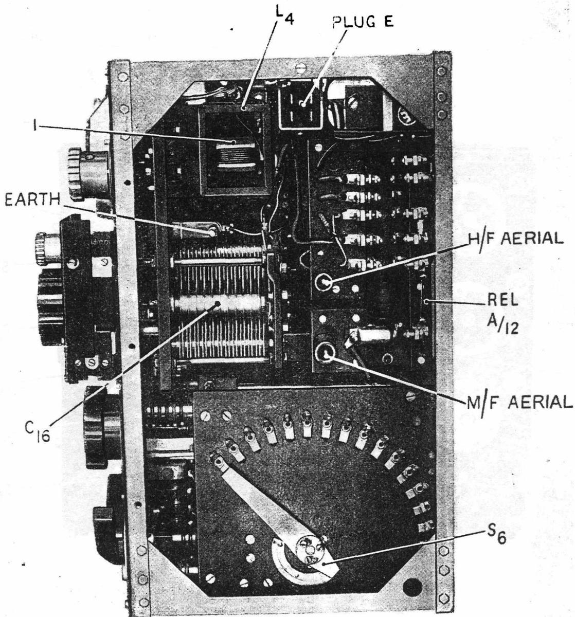
1. Rotor of P.A. tuning variometer, Range 2A
