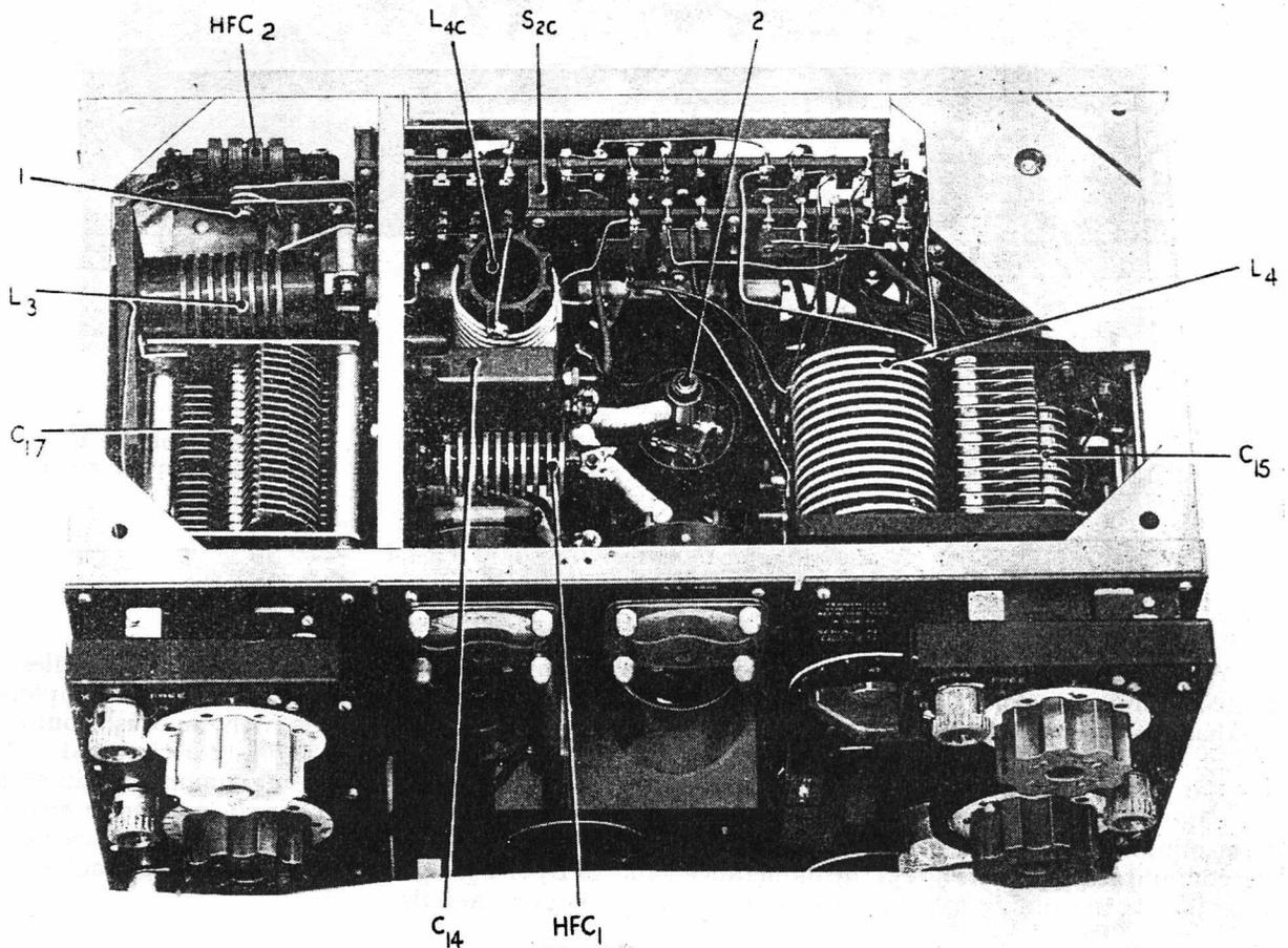
1. Operating crank for  $S_{2c}$       2. Pivoted connector to P.A. valve anode cap
