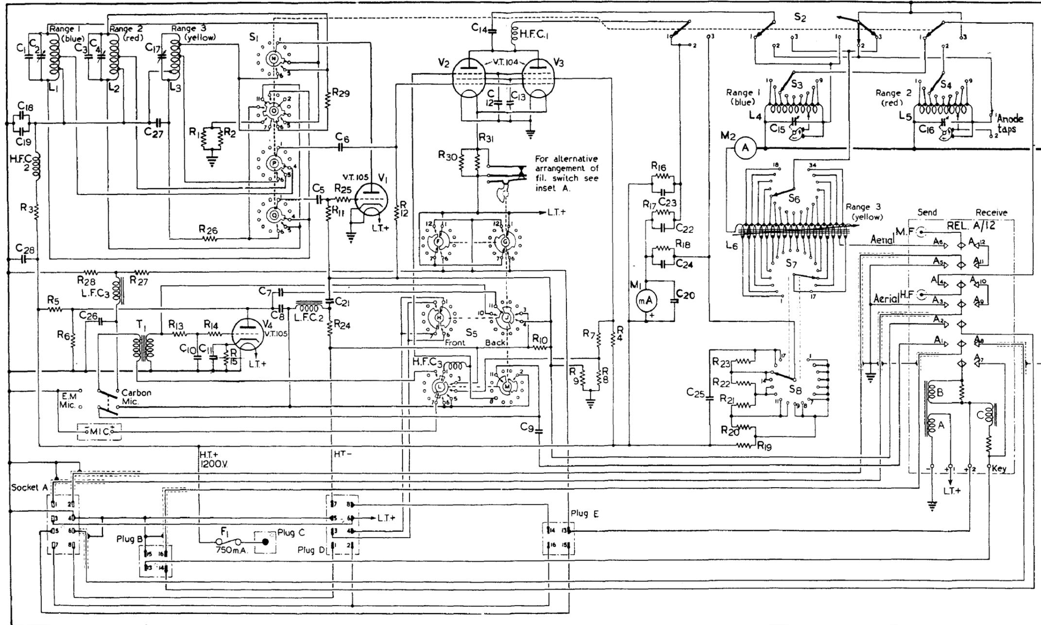
Note. S1 and S5 shown in extreme anti-clockwise position. Socket & plugs as viewed from front of transmitter.
