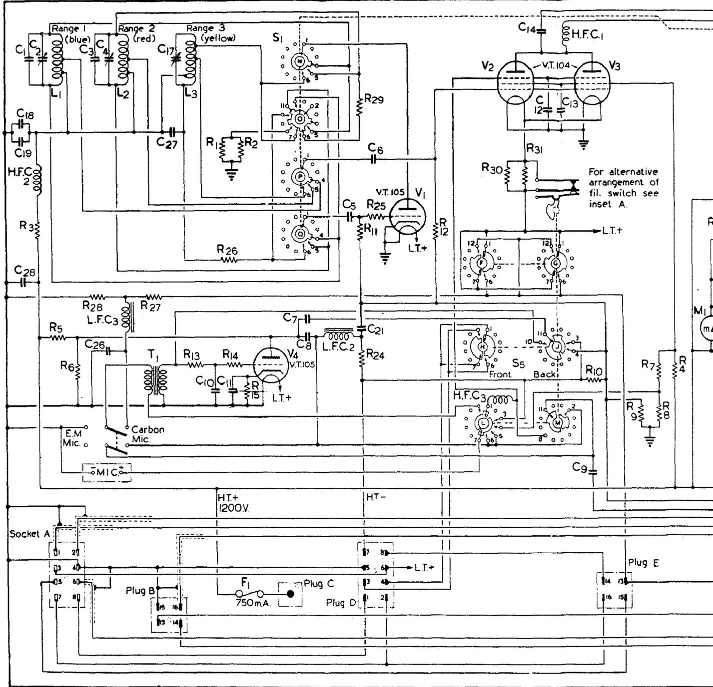
Note. S1 and S5 shown in extreme anti-clockwise position. Socket & plugs as viewed from front of transmitter.
