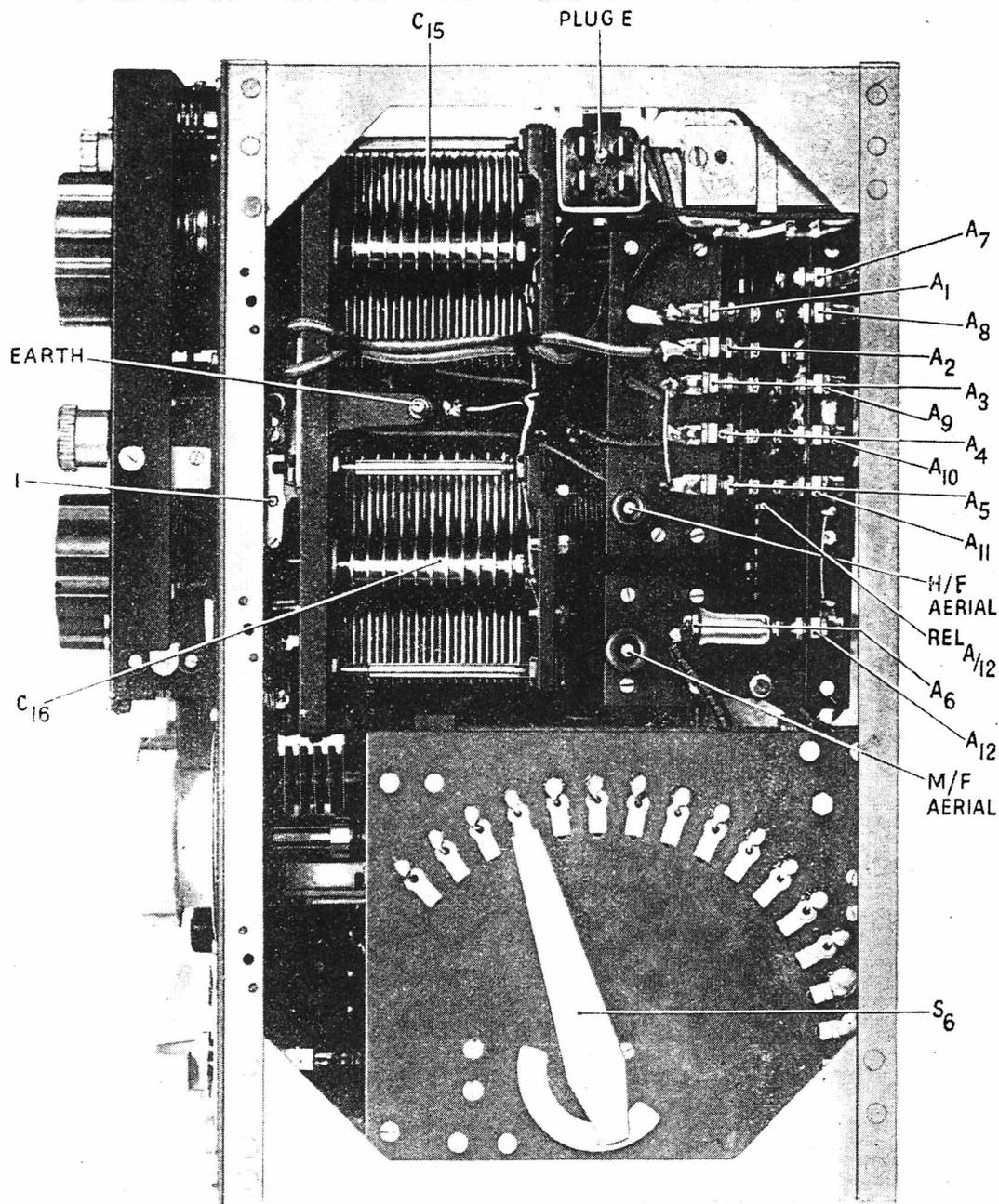
1. Contacts of cam-operated switch on  $C_{16}$
