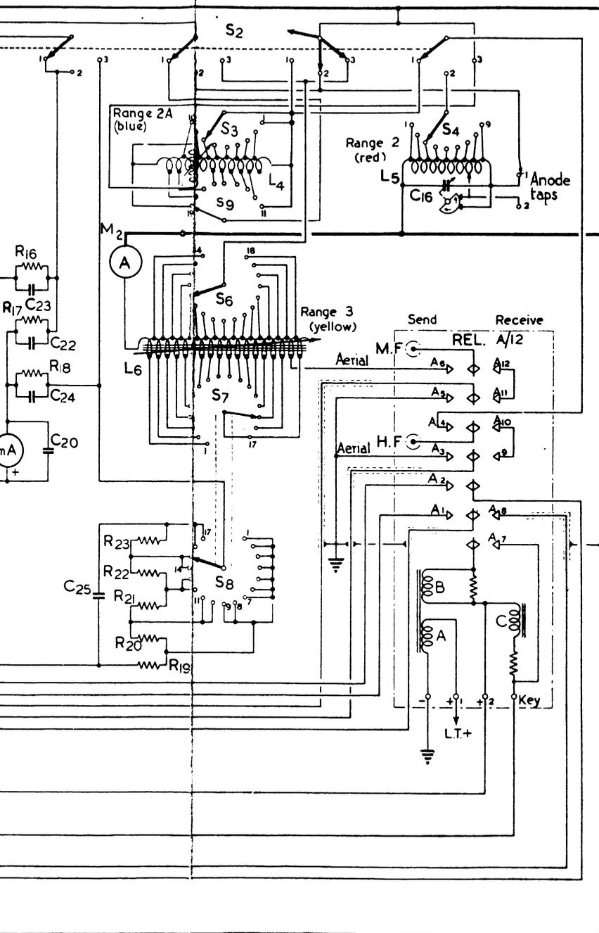
Note. S<sub>1</sub> and S<sub>5</sub> shown in extreme anti-clockwise position.
