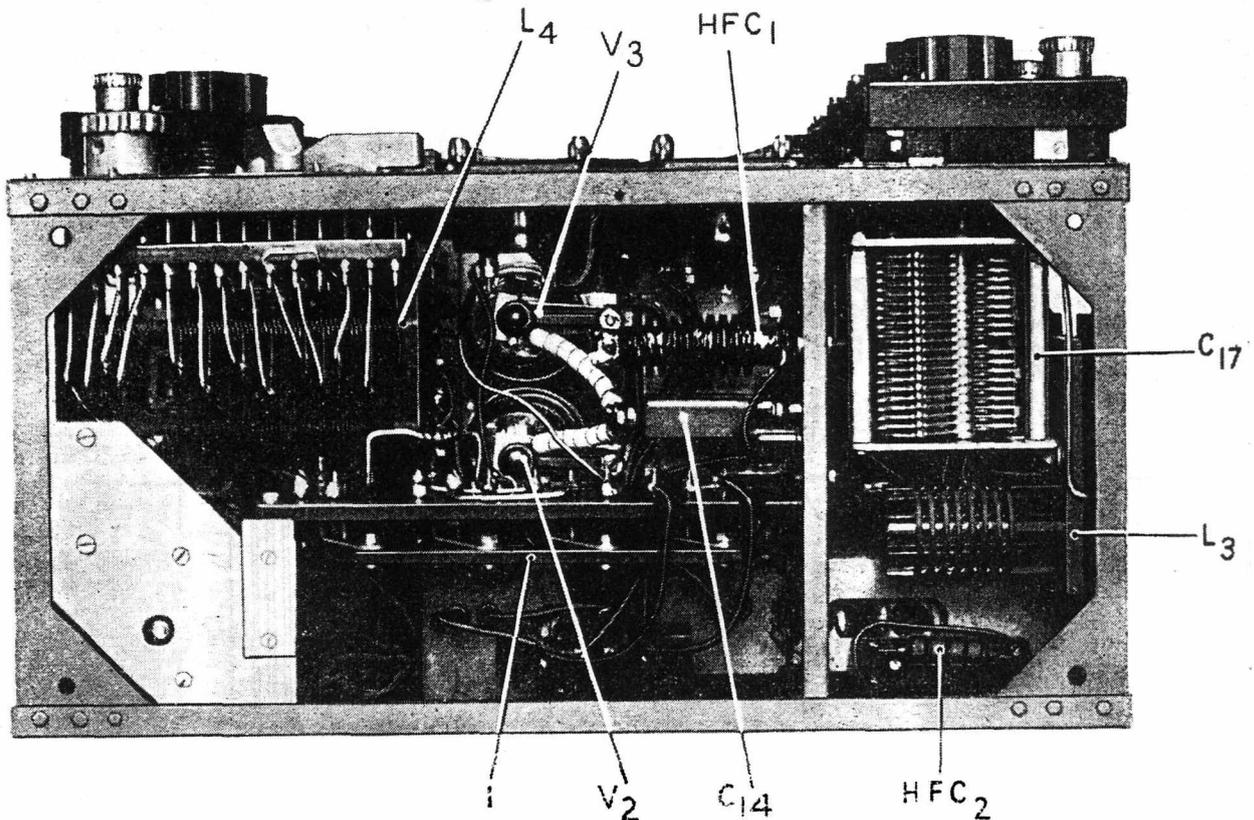
1. Operating bar of four-section frequency range switch
