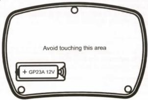
The battery should only be replaced with a high quality battery identical to, or equivalent to an Alkaline GP23A or MN21 12V (10mm diameter x 28mm length). Replacement batteries are available directly from Peak Electronic Design Limited and many good electronic/automotive outlets.
