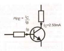
The gain of all transistors can vary considerably with collector current, collector voltage and also temperature. The displayed value for gain therefore
