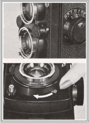
When using the self-timer, always see to it that the Flash Synchronizer Selector is switched to "X" position
