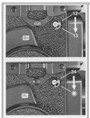
1. When the figure "12" appears in the exposure counter window, it signifies that the full length of the film has been exposed. Another wind of the crank handle will set the exposure counter between "12" and "13", but continue winding until the crank-handle turns freely without tension.
