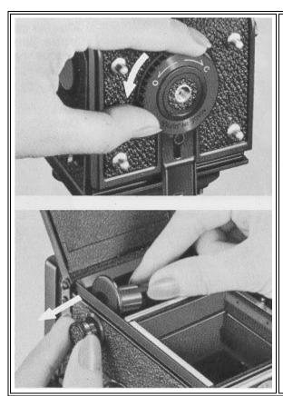
1. The Back Cover will spring open when the Back Cover Locking Ring is turned in the direction of "O" (Open).
