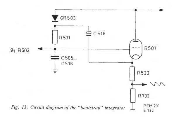
B501' will rise a little, as a result of which the cathode potential rises to the same extent. This voltage rise is applied to the cathode of diode GR503 via capacitor C518, so that the diode is cut-off. The voltage across resistor R531 + R533 thus remains constant.
