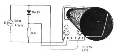
Fig. 10. Displaying the diode characteristic of the OA 85
