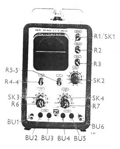
Fig. 26. Front view with adjusting elements
