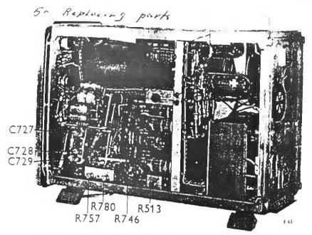
Fig. 24. Right-hand side view adjusting elements and units
