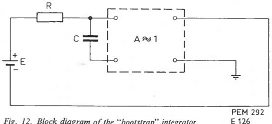
Fig. 12. Block diagram of the "bootstrap" integrator
