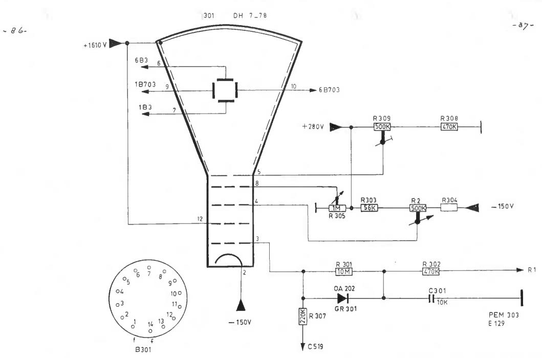
Fig. 35. Diagram of the cathode-ray tube circuit
