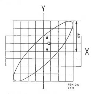
Fig. 7. Determining the phase angles sine  $\varphi = a/b$
