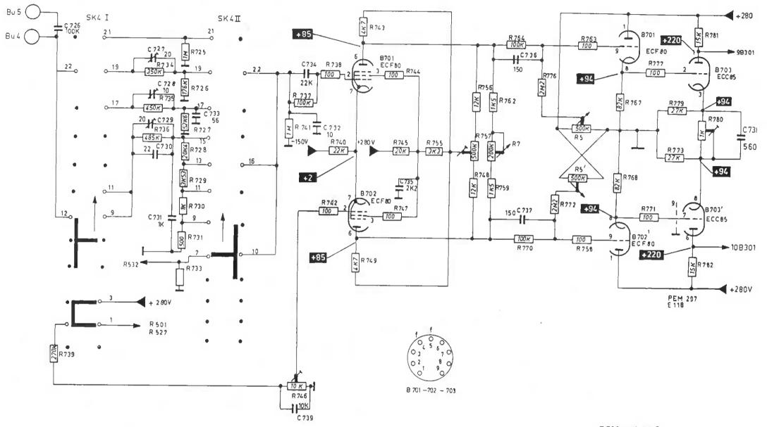
$R733 = 2.7 k\Omega$ R732 is connected in parallel with R733
