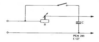
Fig. 8. Network for quadrant determination
