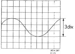
Fig. 5. Measuring the amplitude
