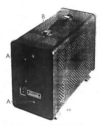
Fig. 14. Removing the cabinet panels
