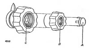
Fig. 15. Removing the knobs
